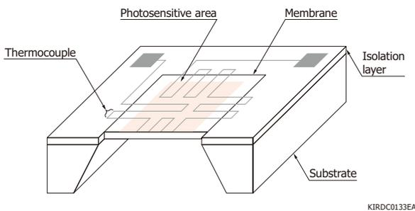
[Figure 2-2] Membrane temperature distribution (uniform incident light) and cross section
