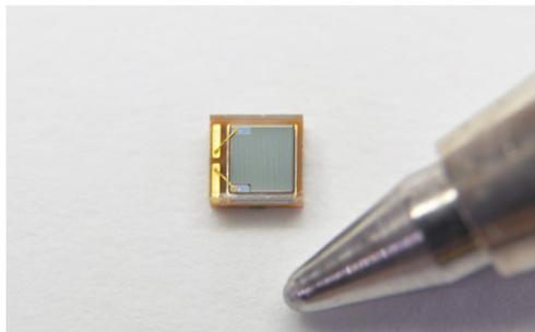
The S15639-1325PS is MPPC for LiDAR applications. The feature is high sensitivity to near-infrared wavelengths.
