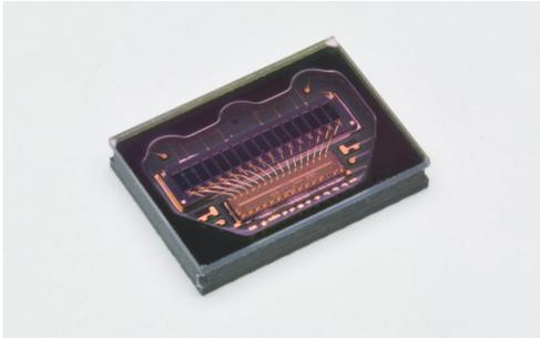
The photosensor with front-end IC is a product packaged with Si APD, which is a typical optical sensor used for TOF, as well as a readout circuit (TIA: trans-impedance amplifier).
