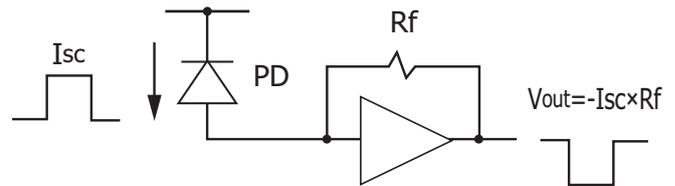
Hamamatsu Photonics provides high-speed low-noise TIAs and proposes photosensor with front-end IC which integrate such as Si PIN photodiode / APD / InGaAs photodiode and TIA in one package. Packaging the detector and TIA into a single device reduces parasitic capacitance and inductance and improves noise and frequency characteristics.
