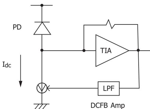
[Figure 3] Band-pass filter implementation example
