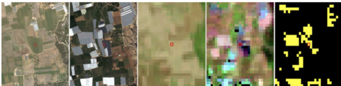
Figure 4.16: Above an example of DIST detection (from [Ying et al. 2017]). The left two panels are two high resolution Google Earth images over the same area in Antalya, Turkey. The next two panels are Landsat acquisitions of the same area. The rightmost panel shows in yellow the vegetation cover loss
