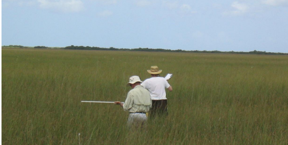
Figure 4.15: Transect-based data collection using an Accupar LP-80 to generate satellite-product relevant [Jones 2011] vegetation cover information for inundated Everglades wet prairie.
